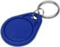
A blue, oval-shaped RFID key fob with a silver metal ring attached to one end.                                                                        | <p>RFID porte clé, type EM4100, 125 kHz</p>                                                                                                                                                                                                                                              |
