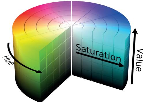
The HSV color model mapped to a cylinder. POV-Ray source is available from the POV-Ray Object Collection.
